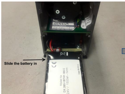
Slide battery assembly in on the guide rail
