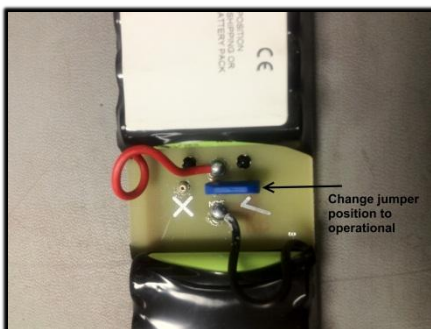
Operational – Enabled Position ✓
