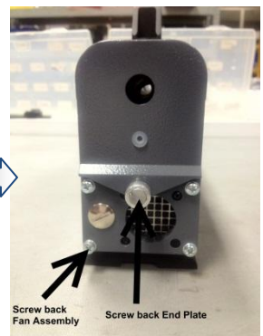
Screw back end plates and top plates as shown
